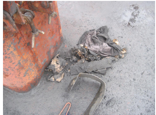
Foreign material, including rags, paper and wood, found in a cargo of iron ore pellets.
