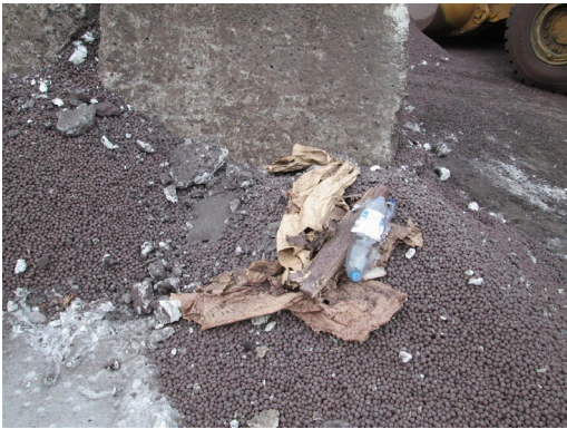
Cargo of iron ore pellets stored in an open area of the Port, contaminated with paper and plastic rubbish.
